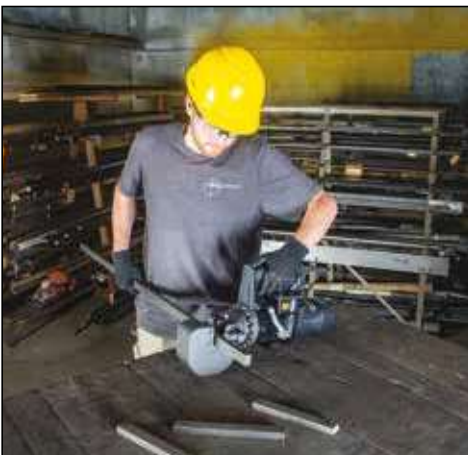
◀ Cutting flat bar is fast and easy with EFBE-Series Electric Flat Cutters.
